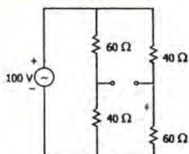
What are the source voltage and source resistance, respectively for the Thevenin's equivalent circuit as seen from the terminals indicated in the circuit given above?
