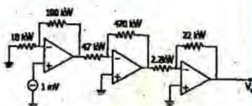
What is the output voltage  $V_o$  of the above circuit?
