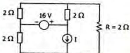
In the circuit shown above, if the current through the resistor  $R$  is zero, what is the value of  $I$ ?
