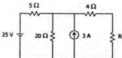
What is the value of  $R$  required for maximum power transfer in the network shown above?
