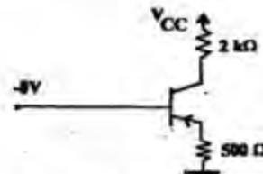
The transistor circuit shown in the figure given above is to function as an amplifier. If  $I_{CQ} = 3$  mA, what is the value of  $V_{CC}$  (approximate)?
