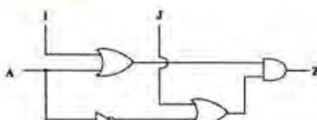
The circuit shown above is to be used to implement the function  $Z = f(A, B) = \bar{A} + B$ . What values are to be selected for I and J?
