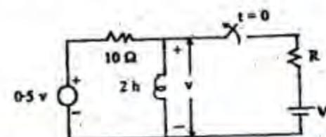
The time constant of the circuit after the switch shown in the figure is opened is
